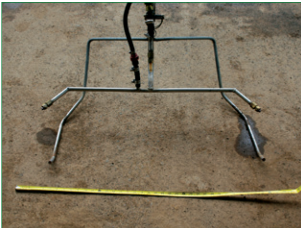
Figure 4 Measuring sprayer width, which can be adjusted to suit row width
