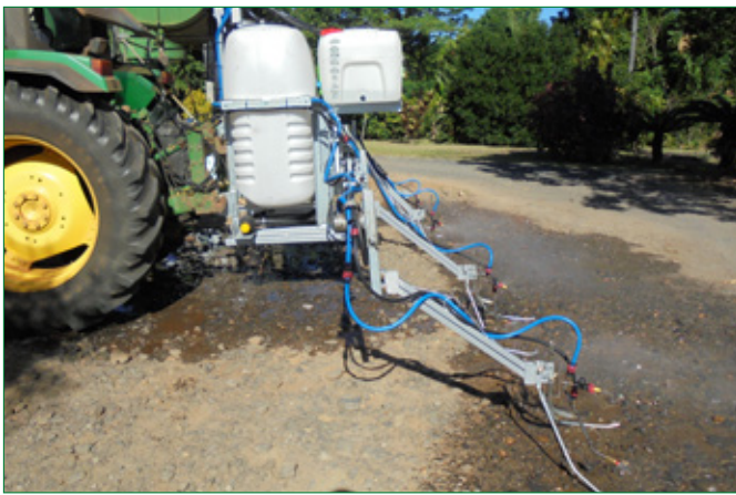
Figure A5.1 The dual herbicide sprayer ready for use
