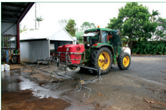
Figure 13 Spray bars being tested after use
