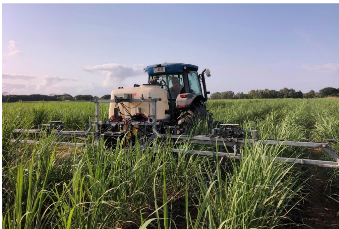
Image 2 Tractor fitted with AutoWeed spraying units during a project trial.
