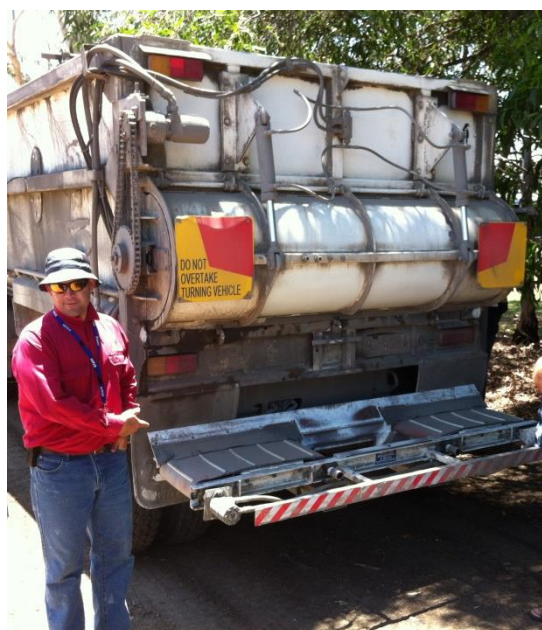
Image 2: Mud cartage truck fitted with a zonal mud applicator
