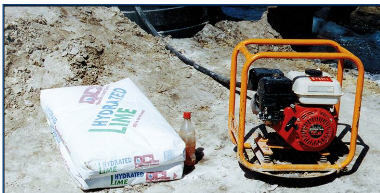
Figure 2 – Hydrated lime can be mixed into slurry and pumped into a pond containing acidic water to neutralise the acid.
